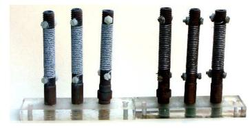
*Figure 5:* Control and CPC treated (Corrosion Block) CLIMAT after exposure at St. Jean Baptiste, Montréal.
